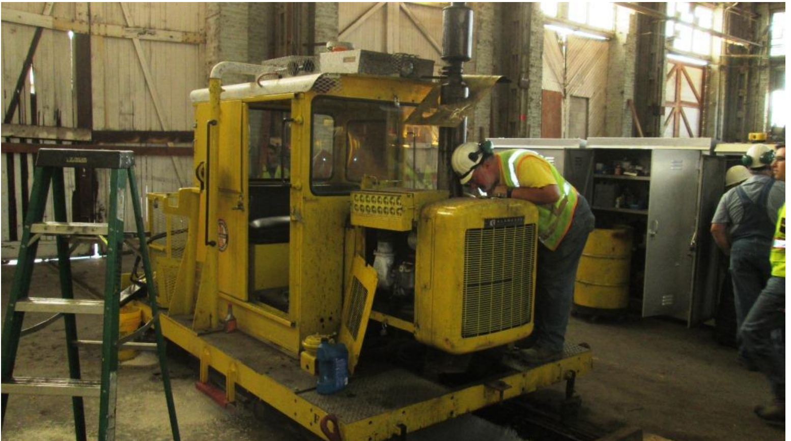
Frank works on removing the bad fan-belts on the Kalamazoo
