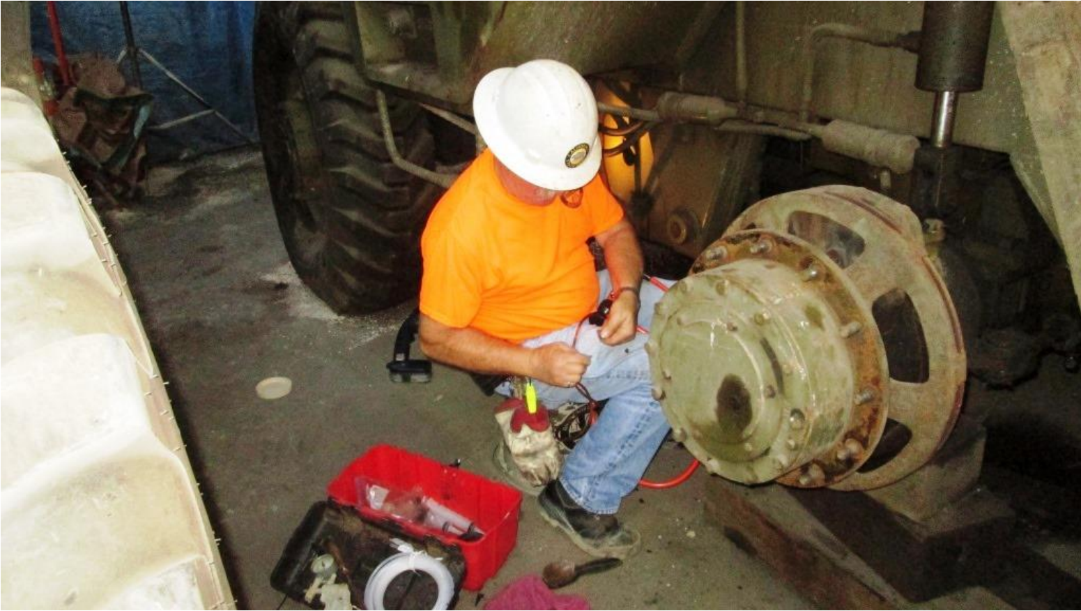
Mike H. siphons dextron out of the second Green Machine's hydraulic transmission
