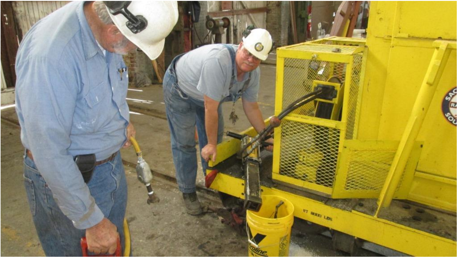
Chris demonstrates the hydraulic spike-puller to Alan
